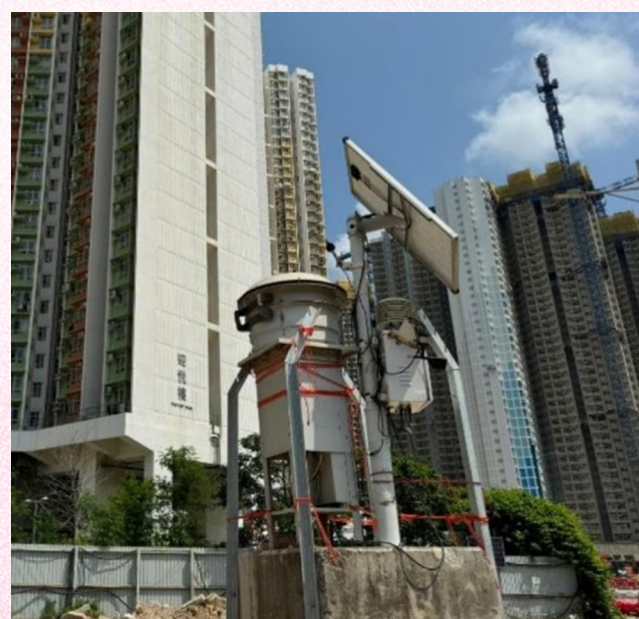
Install dust sensors to monitor air quality in real time 安裝灰塵感應器以實時監測空氣質量
