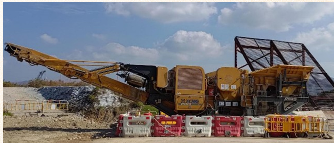
Use of mobile crushing plant to breakdown concrete debris/rock pieces 將移動式碎石機用於輾碎混凝土廢料或石塊
